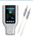
The MVP Icon is an innovative tool used to rapidly assess cleanliness and sanitation in food and beverage facilities. It works by recording the presence of Adenosine Triphosphate (ATP), a molecule found in all living cells such as yeast or bacteria, including those in food and beverage residues.
