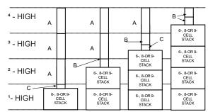
Adapter combinations are the same for the 13" and 16" or 6", 8" and 9" cell stacks regardless of dome height or housing style.
