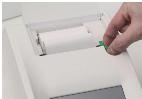
Pull down the green lever to secure the printing roll and turn the green wheel to adjust the paper.
