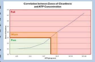
are not truly dirty until the level of ATP reaches approximately 16-50 picograms. If desired, the Pass, Warn and Fail thresholds can be adjusted to suit a specific environment or hygiene monitoring goal, based on a user's own internal validation.
