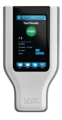
by the MVP ICON instrument. The amount of light emitted is directly related to the amount of ATP present in the sample. This allows the MVP ICON to instantly determine if a surface is sufficiently clean or if it is dirty and should be re-cleaned to prevent possible contamination of the product.
