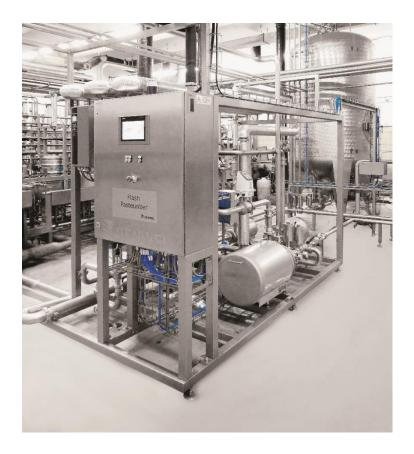
Pasteurization is a heat treatment with the purpose of improving the microbiological stability of the beverage in order to prolong its shelf life. While reducing the number of harmful microorganisms, uniform and gentle treatments are required to maintain the original taste and appearance of the beverage.
