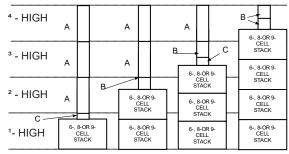
Adapter combinations are the same for the 13" and 16" or 6", 8" and 9" cell stacks regardless of dome height or housing style.
