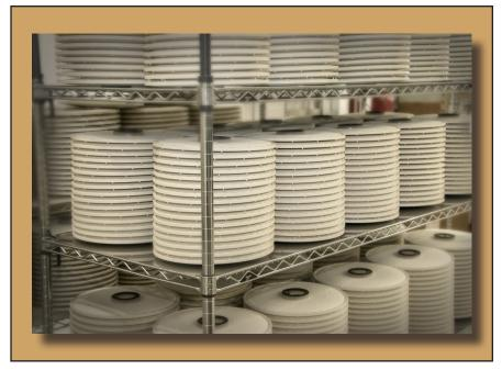
Cellu-Stack filters are designed for ease in loading and unloading filter housings. This significantly reduces operating costs and production downtime.
