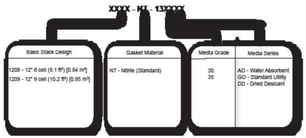
Example: To order a 9 cell 1330 Utility Series 12" 1330 Cellu-Stack® filter with nitrile gaskets in an AO series, the order should read as follows: 1209-NT-1330AO.
